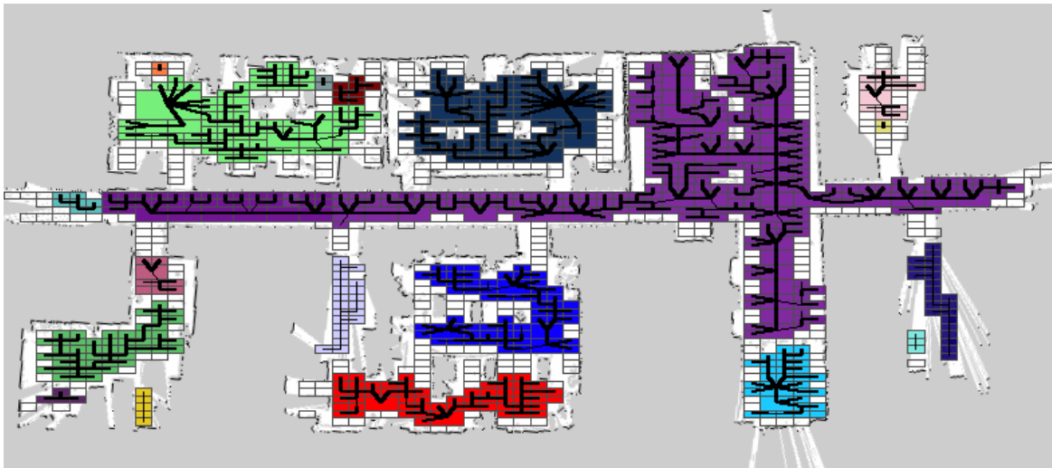
(b) Segmentation by mutual information at th = 1.6 . The noisy small regions can be eliminated by median filters
