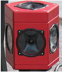
Figure 3: Ladybug 3 with 5 cameras placed horizontally in circle and one camera looking upwards for capturing omnidirectional images.
