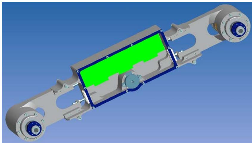
**Figure 6. Mechanical base of the bogie**
